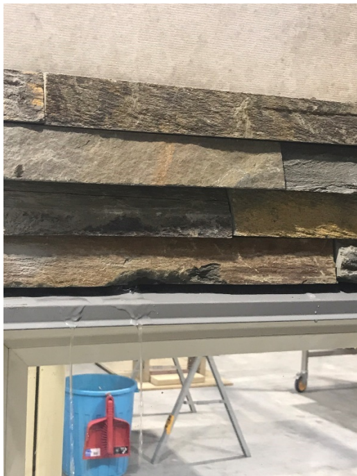
Figure 9. Water management test above the window head flashing.
